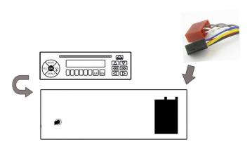
Finally, connect the female ISO and the mini-ISO plugs to the corresponding connectors in the vehicle
